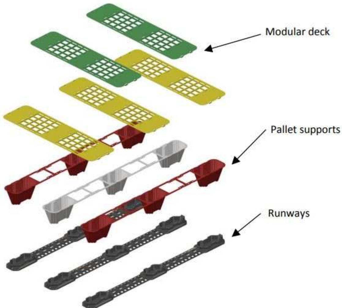
Depending on customer needs, **Topy Pallet System** makes it possible to adapt different types of plastic structure in order to be able to support various types of products. An advantage that makes this product extremely competitive is the price. This combination is extremely cheap.
